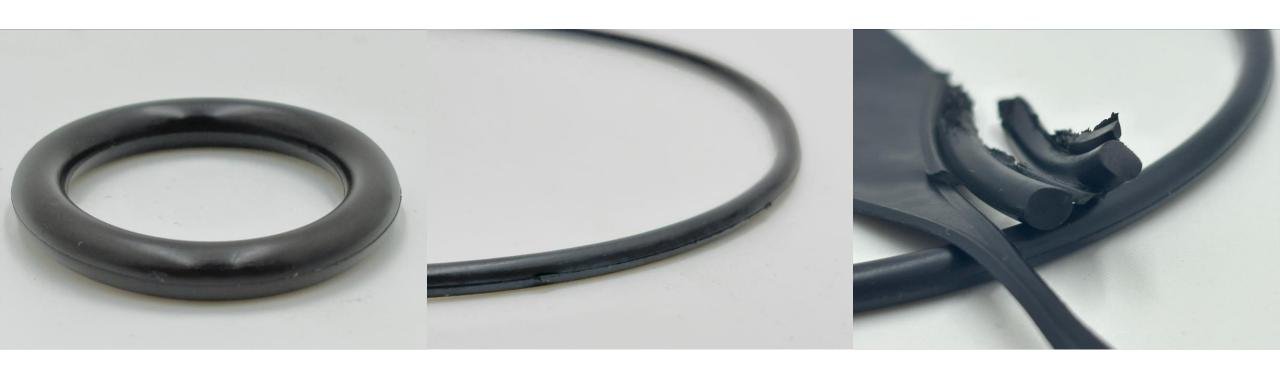
As you can see, O-rings made entirely from FKR-2275UP can be molded to standard specifications. The interior of the O-ring is solid with no issues, and its performance is similar with Virgin FKM. However, there is a higher probability of burrs forming on the appearance. If filled with 60% to 80%, the appearance will be indistinguishable from Virgin FKM.
